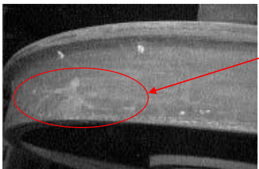
Fig. 9 Major irregular crushing of the edge of the tyred wheel rim
