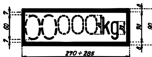
Figure 2: Wagon tare and braked weight of the platform-operated hand brake
